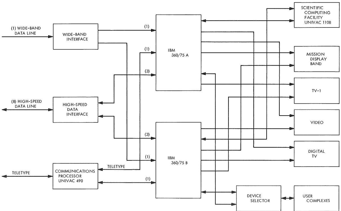
**Fig. 2. SFOF Mariner Mars 1971 IBM 360/75 computer configuration**
